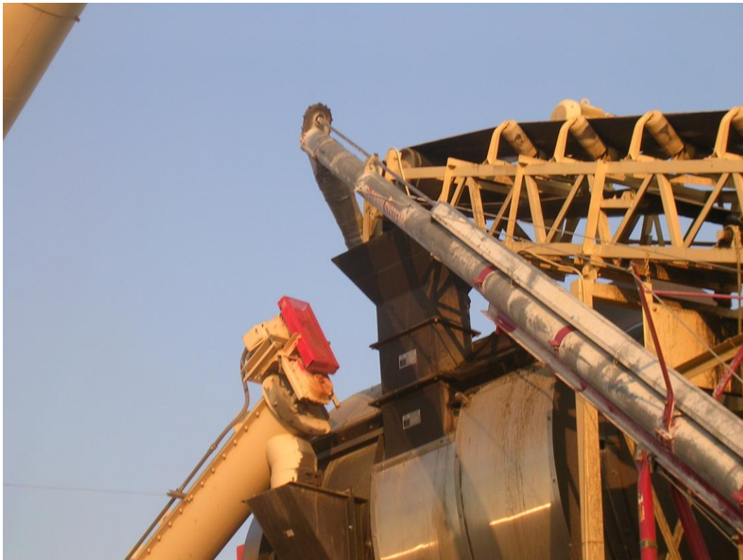
Photo 2 Blended Crumb Rubber/TOR Being Added To Plant at RAP Collar
