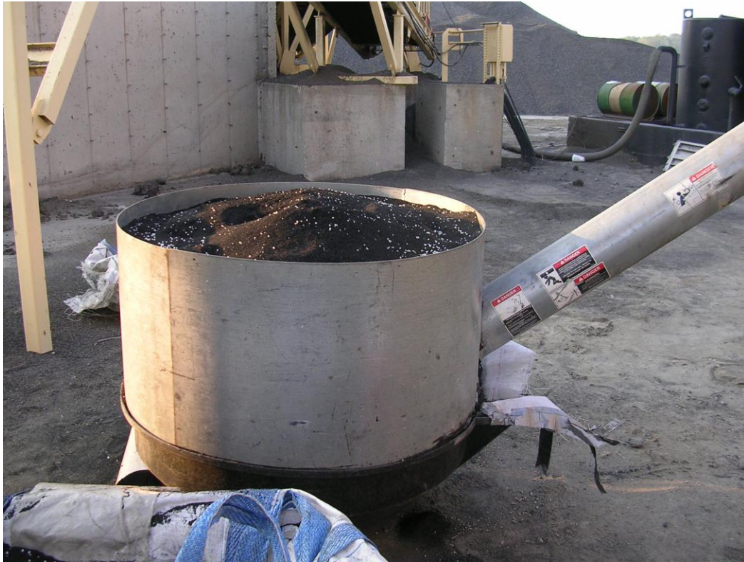
Photo 1 Blended Crumb Rubber/TOR Feeder Container
