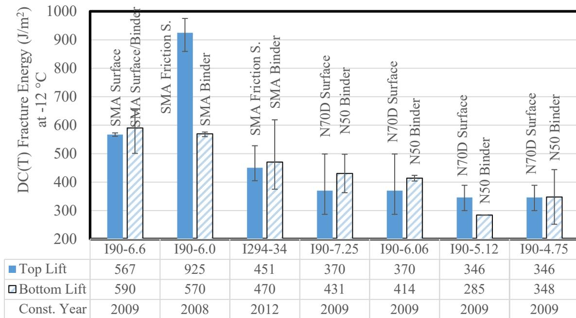
Figure 5-2. Comparing fracture energies for top and bottom lifts of the field cores
