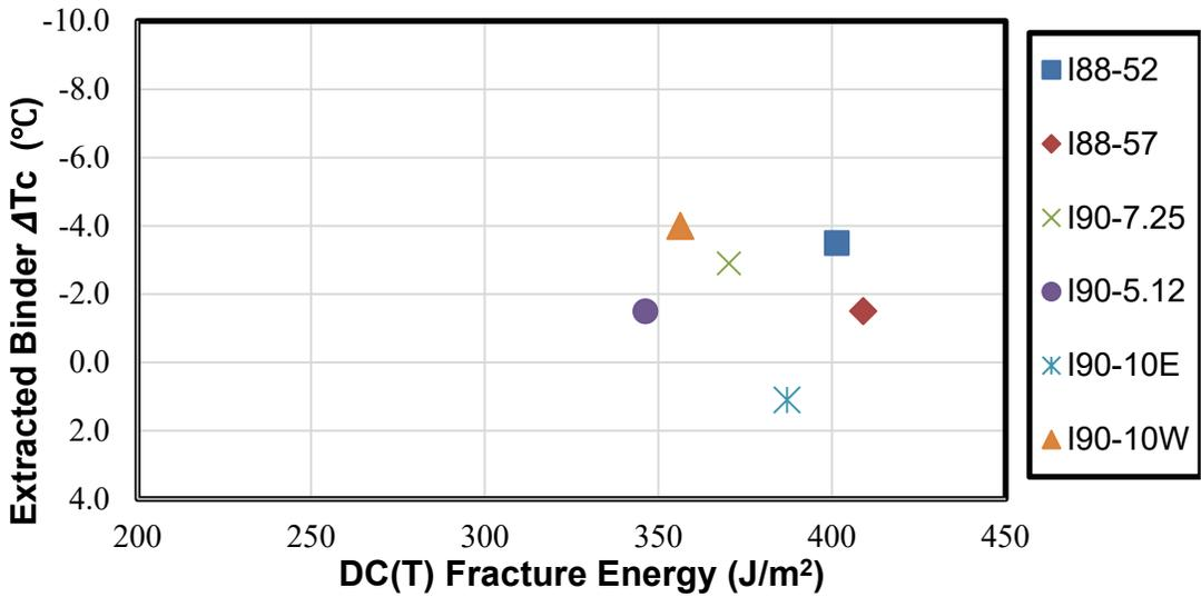
Figure B-6. Comparison between DC(T) fracture energy and extracted binder  $\Delta T_c$  for field cores
