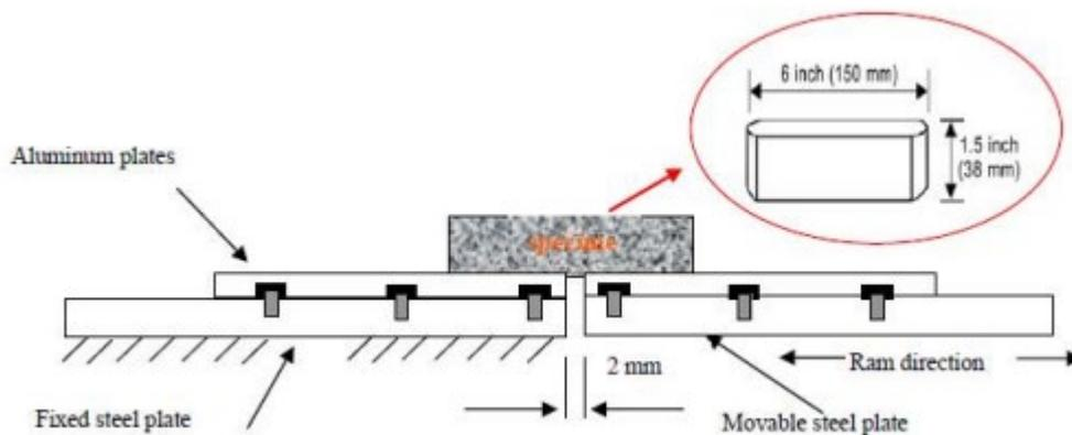
Figure A-5. Concept of Overlay Test (Fujie Zhou, Scullion, & Hu, 2007)
