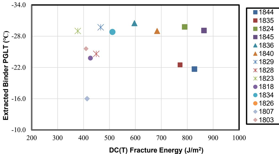
Figure B-1. Comparison between the DC(T) fracture energy and extracted binder PGLT
