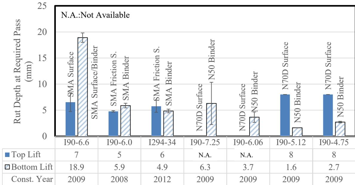
Figure 5-9. Comparing the rut depths for top and bottom lifts of the field cores
