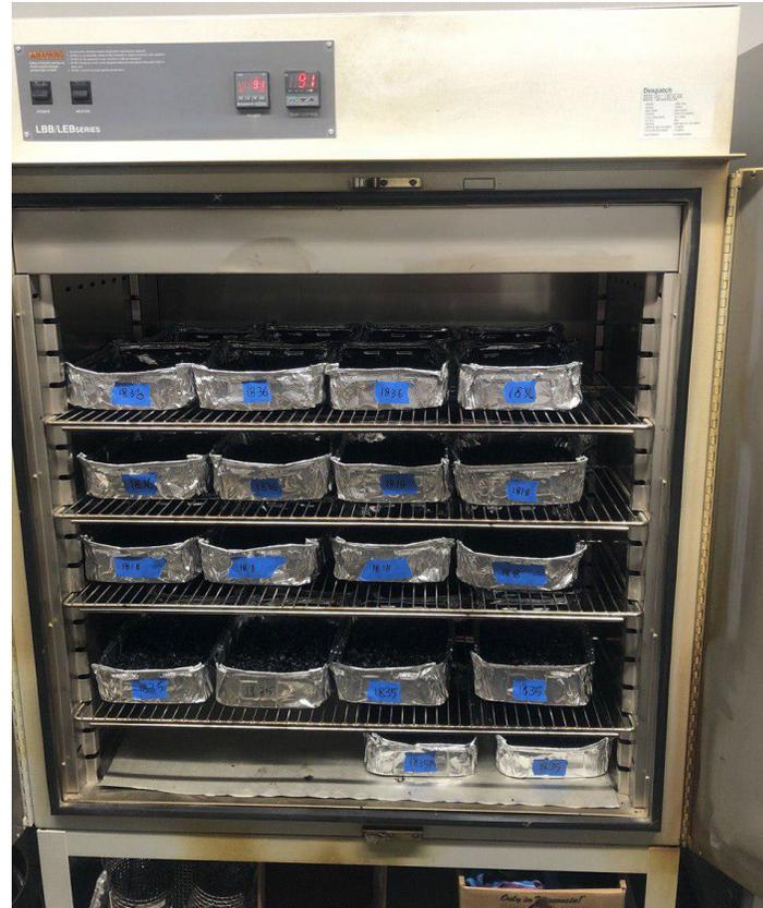
Figure 3-21. Aging the Tollway 2018 plant produced mixtures in oven at 95 °C for 6 days
