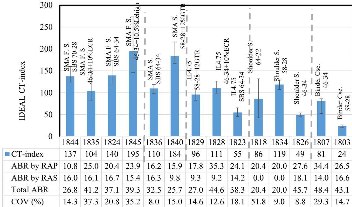
Figure 3-8. Results from IDEAL-CT testing (95 mm sample thickness)
