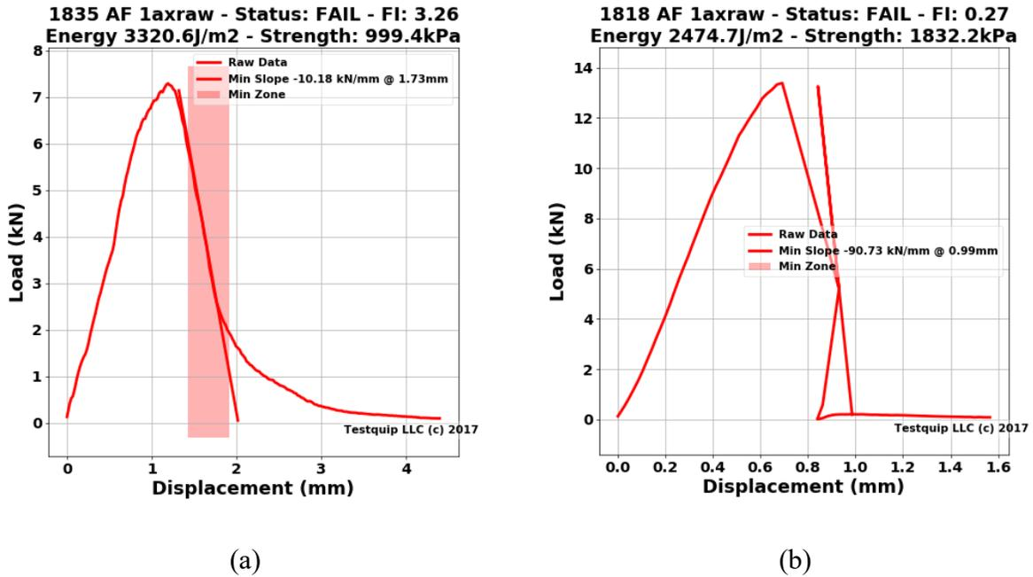
Figure 3-24. Load-displacement response for aged mixtures under I-FIT testing: a)1835
