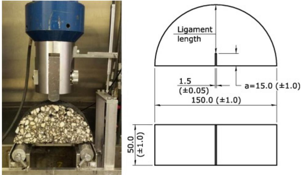
Figure A-3. SCB specimen and test setup (Ozer, Al-Qadi, et al., 2016)
