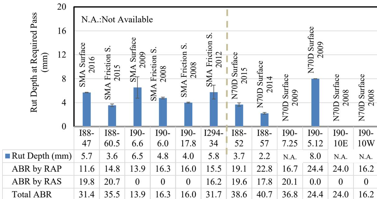
Figure 5-8. Hamburg testing results for the top lift of the field cores
