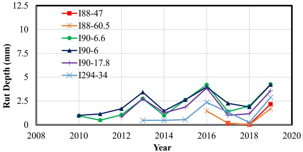
Figure 6-8. Comparison of rut depth values vs. year in service
