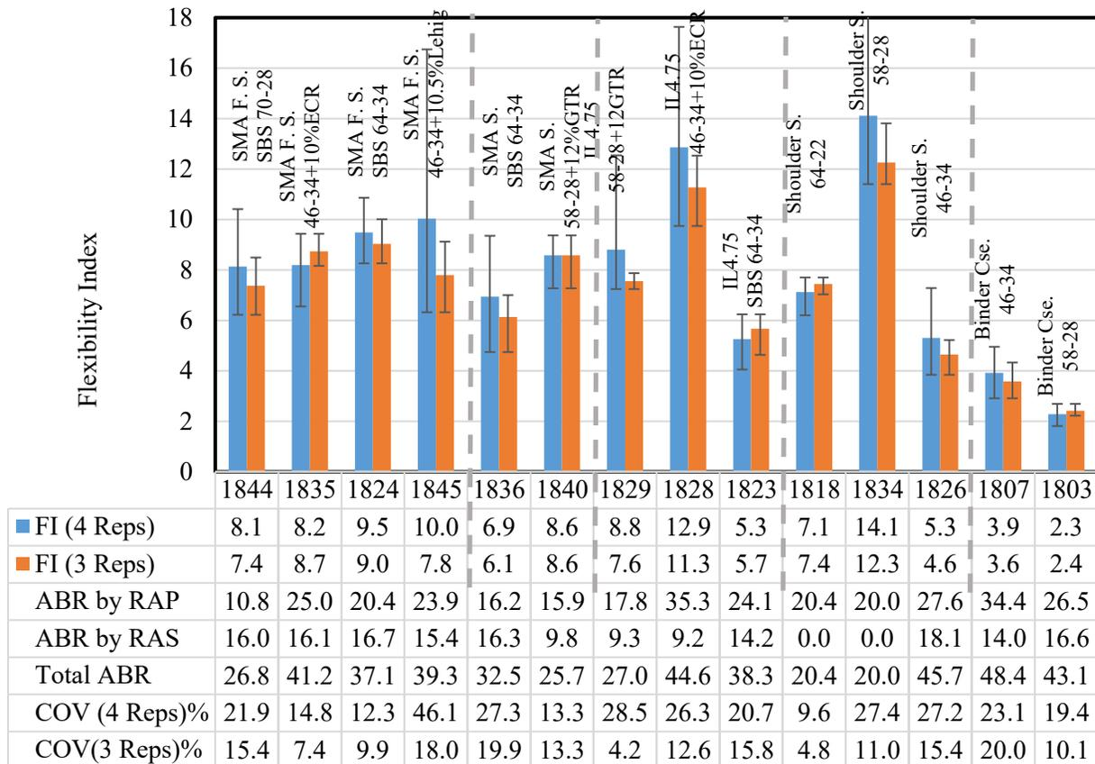
Figure 3-5. I-FIT testing results (four replicates vs. three replicates)
