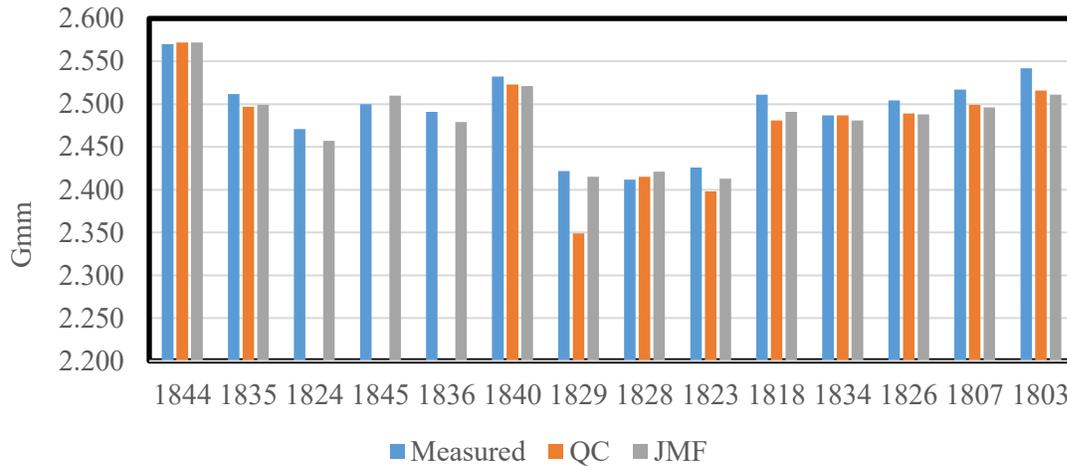
Figure 2-7. Comparing different  $G_{mm}$  values for the studied mixtures (Measured = Test performed in MAPIL; QC = Measured by quality control crew; JMF = job mix formula)
