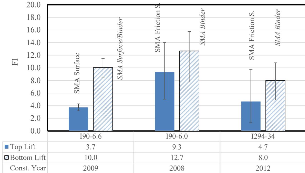
Figure 5-4. Comparing the FIs for top and bottom lifts of the field cores
