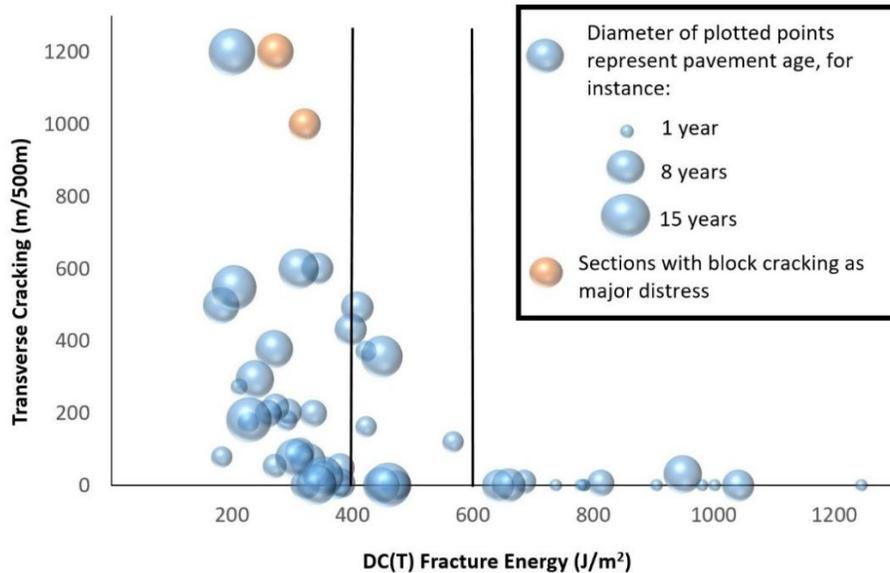
Figure 7-1. Transverse cracking vs. DC(T) fracture energy (Buttler et al., 2018)
