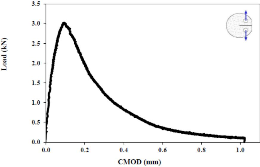
Figure A-2. Typical Load-CMOD curve (W. G. Buttlar & Wang, 2016)
