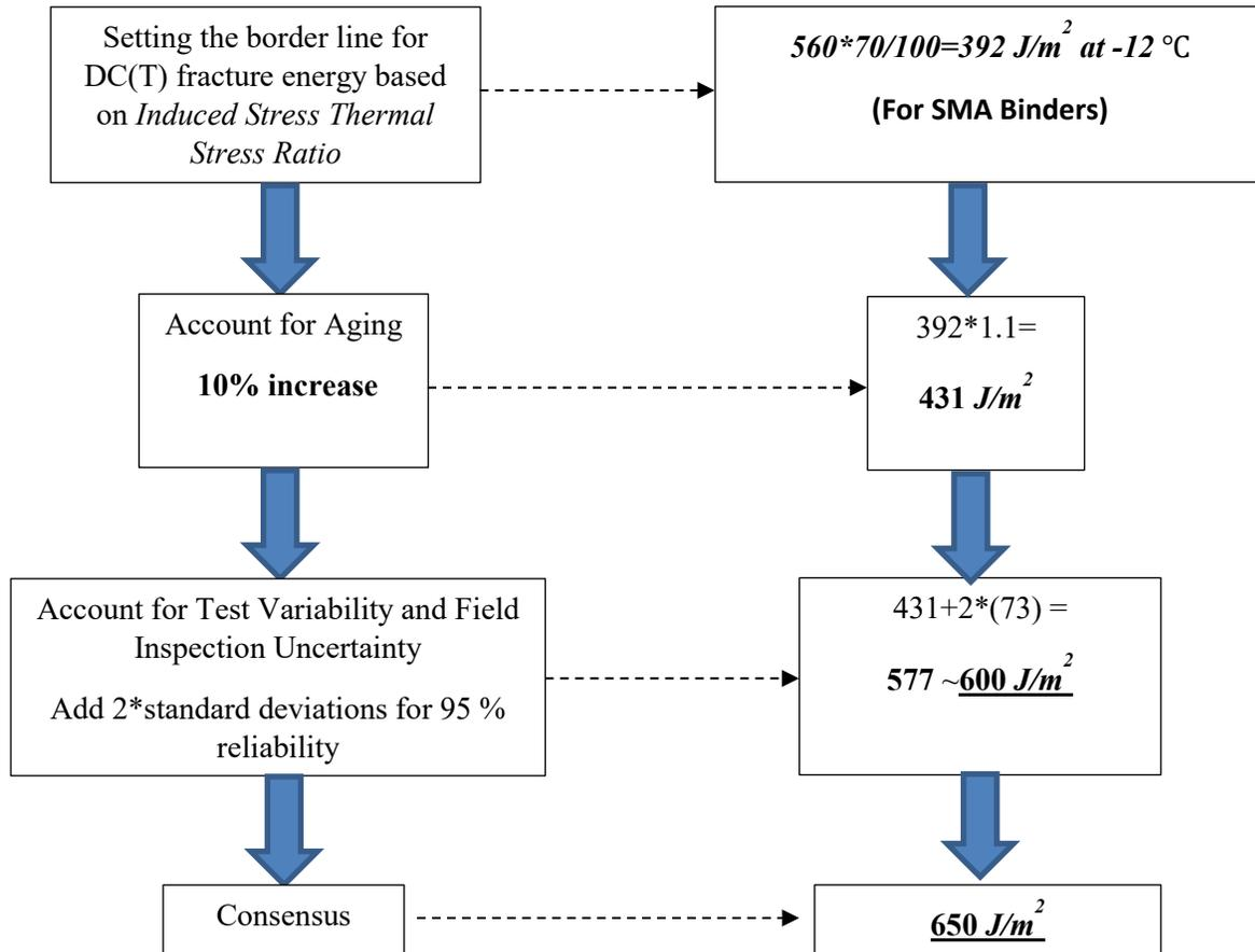
Figure 7-11. Flowchart to Calibrate DC(T) spec for SMA binder mixtures
