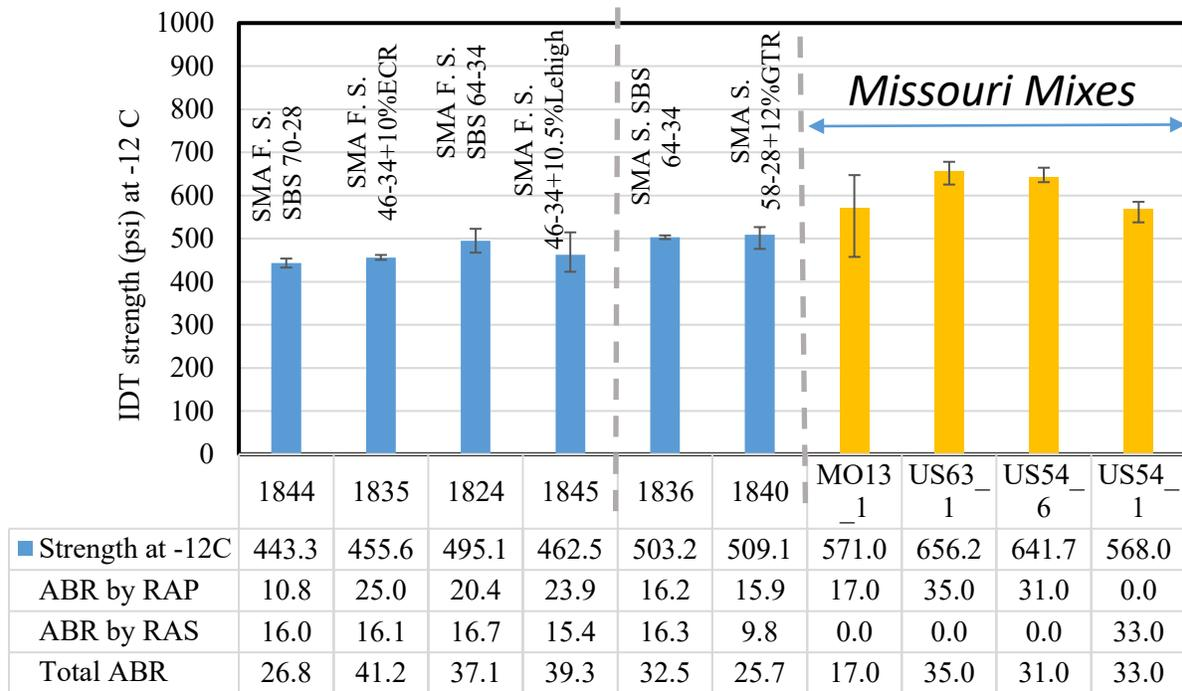
Figure 3-9. IDT strength testing results at -12 °C
