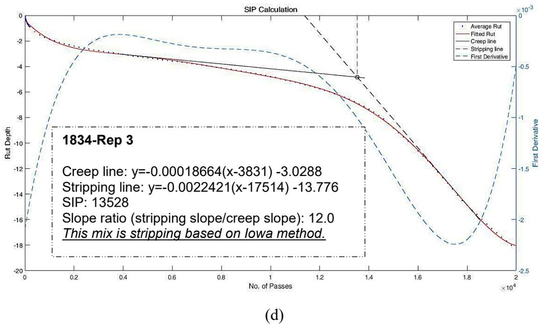
Figure 3-13. Examples of determination of SIP: a) 1835, b) 1845, c) 1828, d) 1834 mixtures
