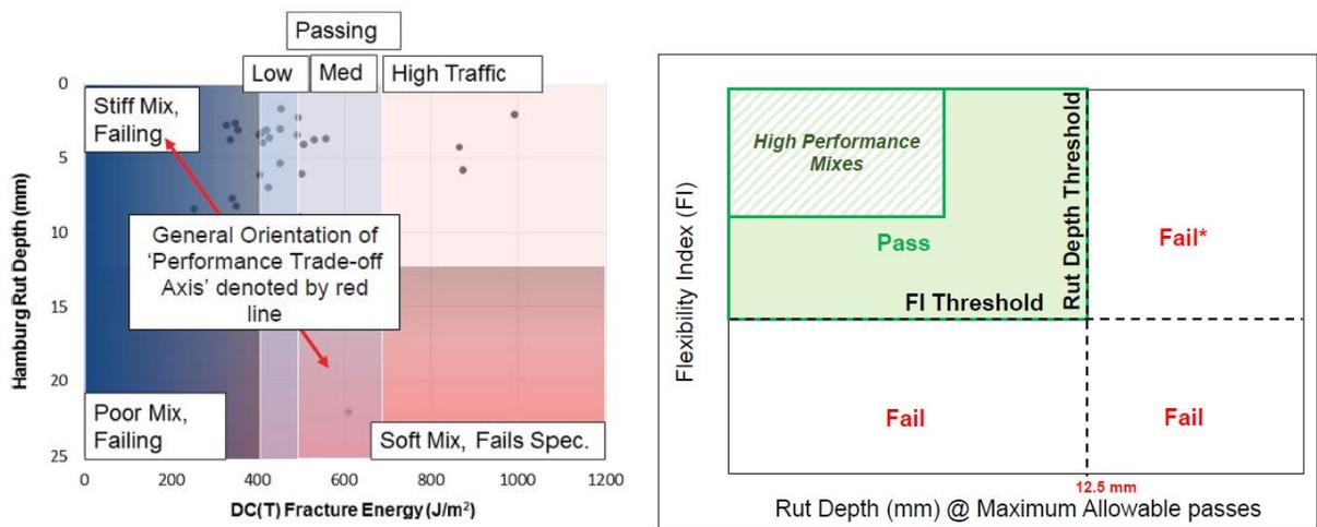
Figure A-9. a) Performance-Space diagram with limits superimposed (W. G. Buttler et al., 2016) b) Interaction plot for a balanced mix design (Al-Qadi et al., 2015)
