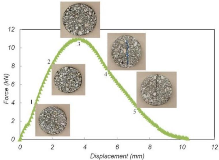
Figure A-6. IDEAL-CT Test Setup and Typical Results (Fujie Zhou et al., 2017)
