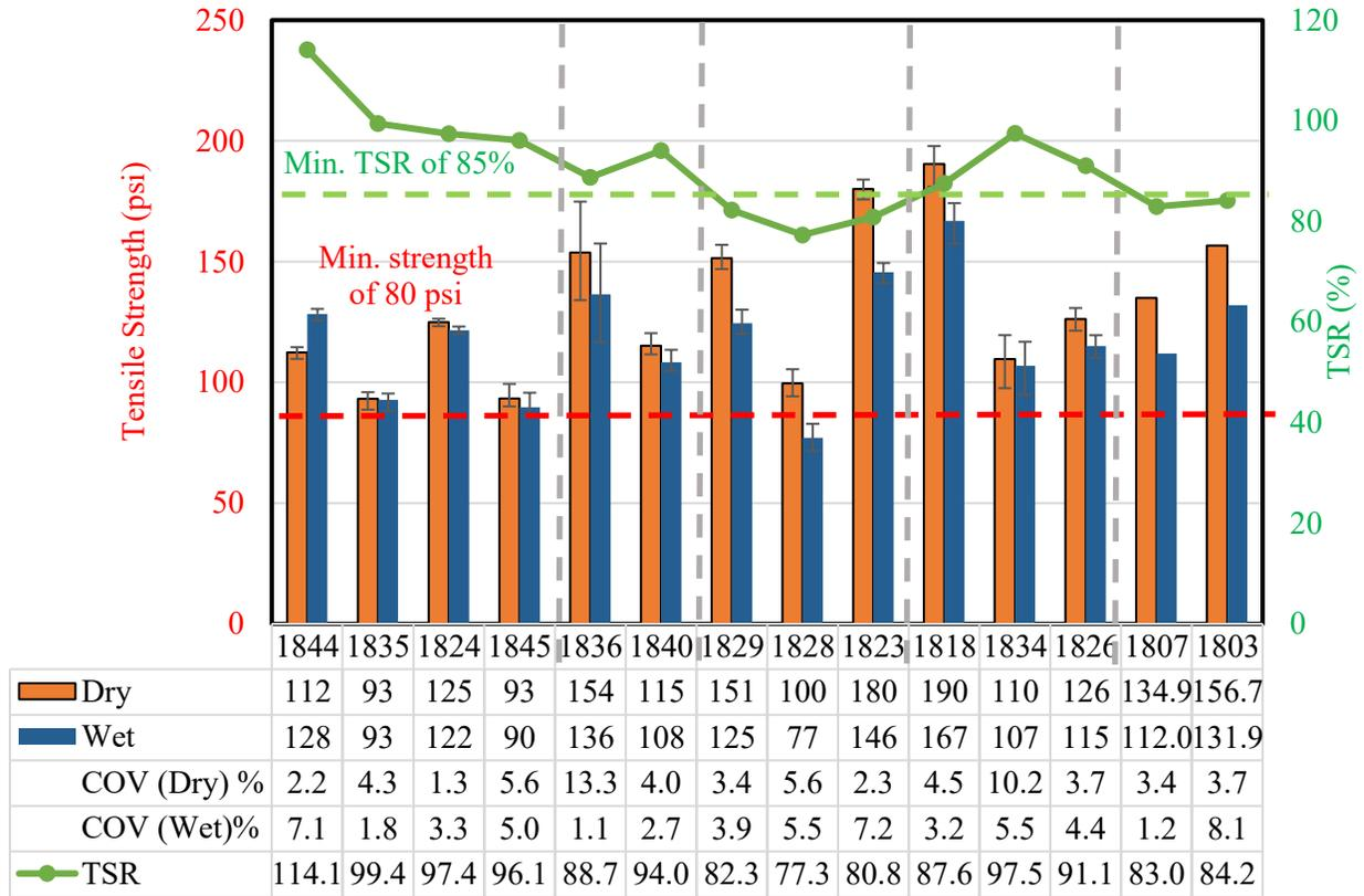
Figure 3-16. Wet and dry strengths and TSR values
