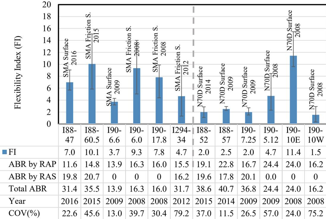
Figure 5-3. I-FIT testing results for the top lift of the field cores
