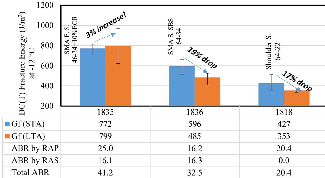
Figure 3-22. Comparing the DC(T) fracture energies of short-term aged (STA) with long-term aged (LTA) samples
