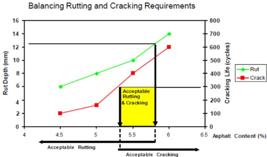
Figure A-13. Balance of Rutting and Cracking Developed in Texas Study (F. Zhou et al., 2014)
