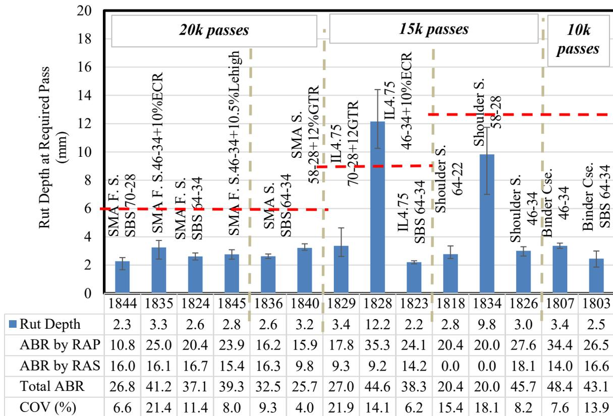
Figure 3-11. Hamburg testing results at required number of passes at 50 °C
