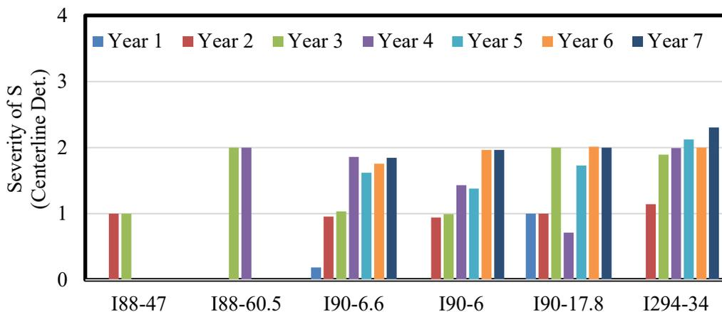
Figure 6-3. Average severity of centerline deterioration distress (S) as a function of service life
