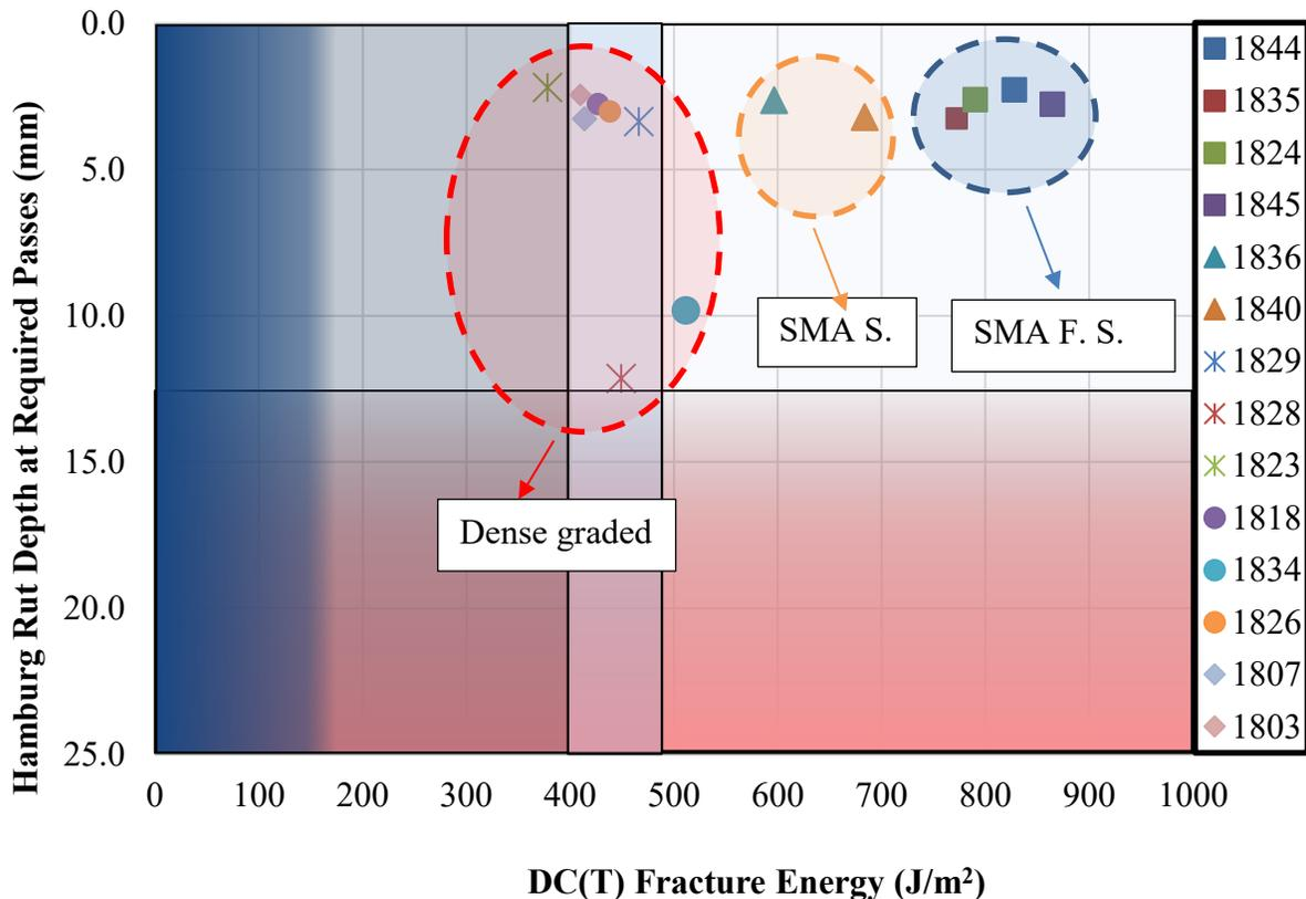
Figure 3-19. Hamburg-DC(T) performance-space diagram for 2018 mixtures
