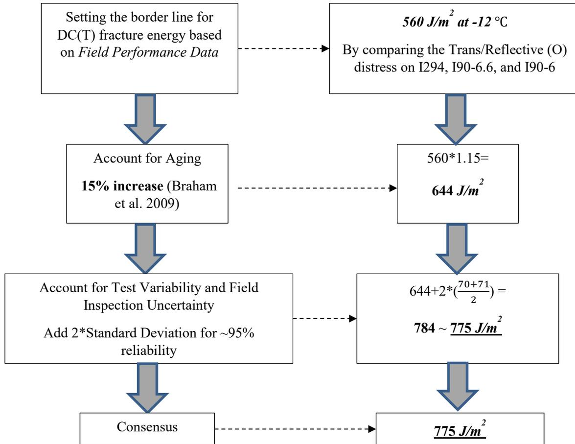
Figure 7-9. Flowchart to Calibrate DC(T) spec for SMA friction surface mixtures
