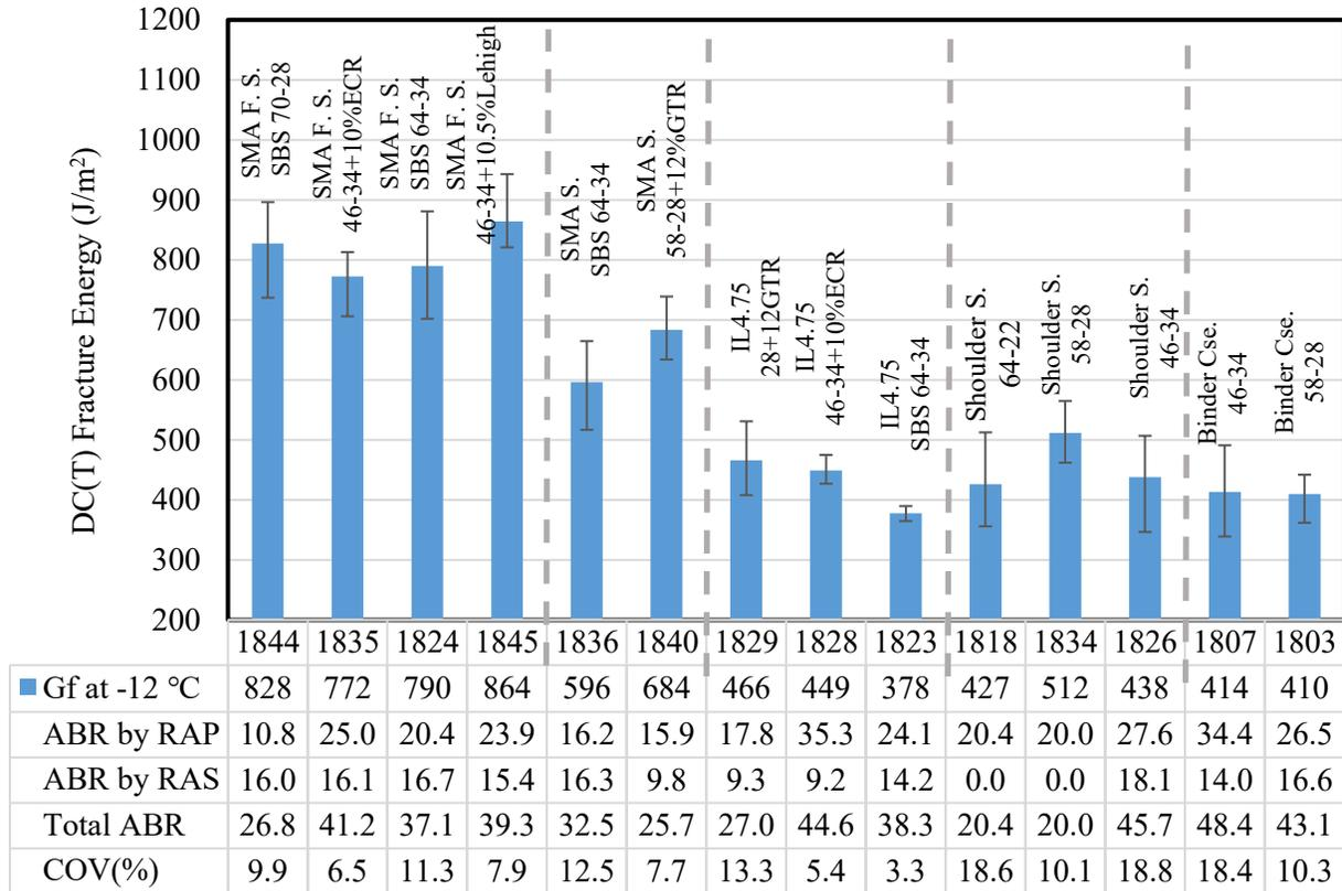
Figure 3-1. DC(T) fracture energy at -12 °C using MAPIL samples
