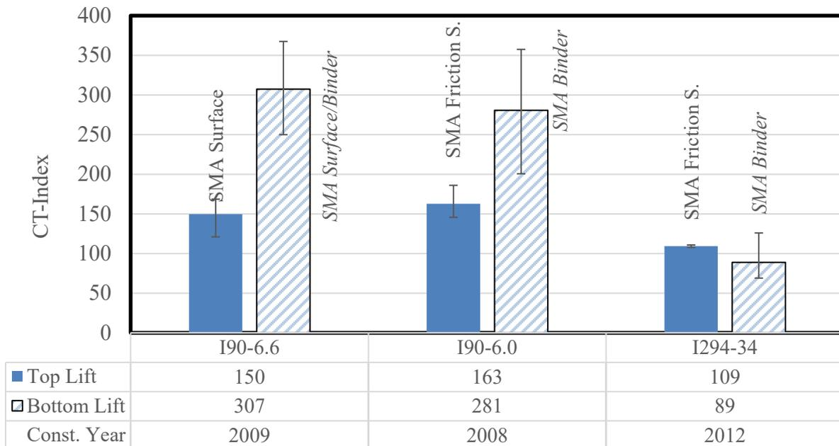
Figure 5-6. Comparing the IDEAL-CTs for top and bottom lifts of the field cores
