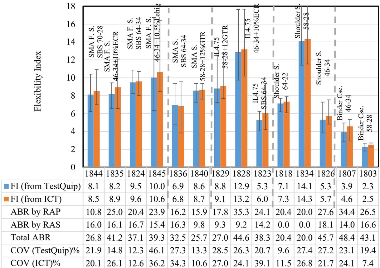
Figure 3-7. Comparing FIs calculated from Test Quip and ICT software
