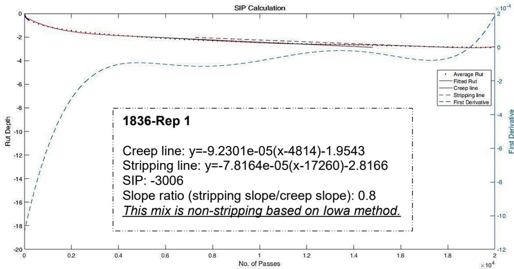
Figure 3-14. Parallel creep and stripping lines for 1836 mix.
