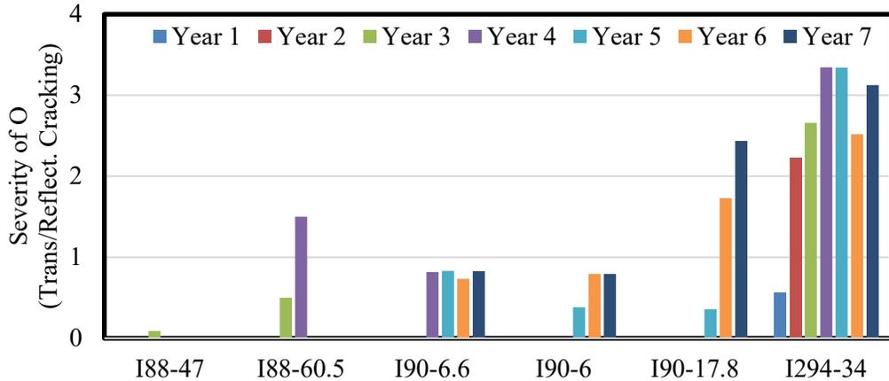
Figure 6-5. Average severity of transverse/reflective cracking distress (O) vs. service life
