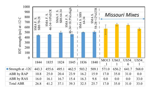
Figure 3-9. IDT strength testing results at -12 °C
