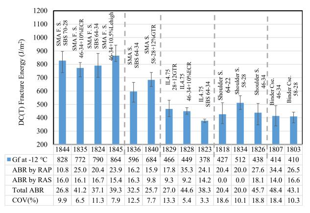
Figure 3-1. DC(T) fracture energy at -12 °C using MAPIL samples
