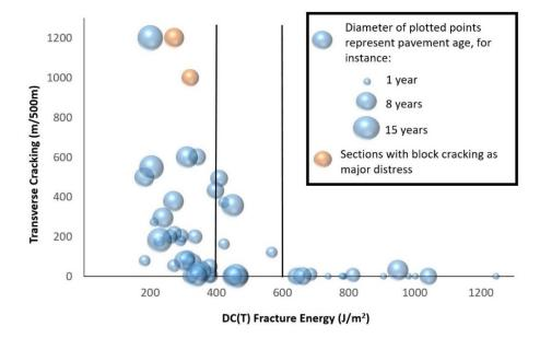
Figure 7-1. Transverse cracking vs. DC(T) fracture energy (Buttlar et al., 2018)
