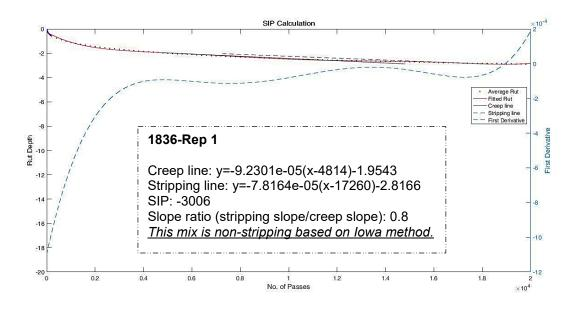
Figure 3-14. Parallel creep and stripping lines for 1836 mix.
