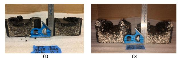
Figure 3-12. Tested samples after 20K pass at 50 °C. a) 1828 mix, b) 1834 mix
