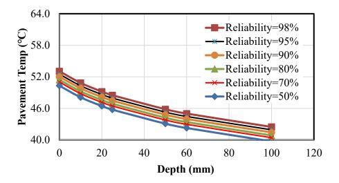
Figure 7-6. LTPP bind software outputs for pavement temperature in summer as a function of depth and reliability in Northern Illinois
