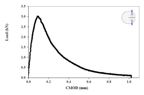
Figure A-2. Typical Load-CMOD curve (W. G. Buttlar & Wang, 2016)
