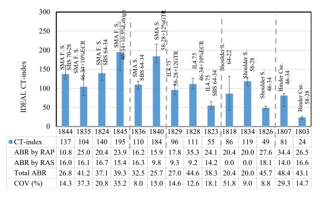
Figure 3-8. Results from IDEAL-CT testing (95 mm sample thickness)
