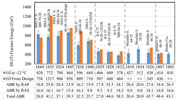
Figure 3-2. Comparing DC(T) fracture energy at -12 °C: current study vs. JMF
