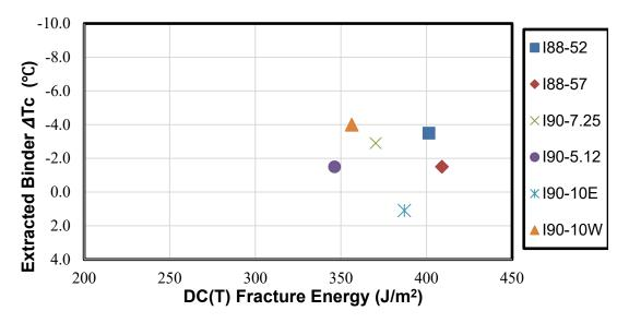
Figure B-6. Comparison between DC(T) fracture energy and extracted binder  $\Delta$ Tc for field cores
