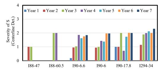
Figure 6-3. Average severity of centerline deterioration distress (S) as a function of service life
