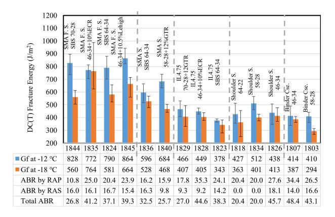
Figure 3-4. Comparing DC(T) fracture energy at -12 and -18 °C
