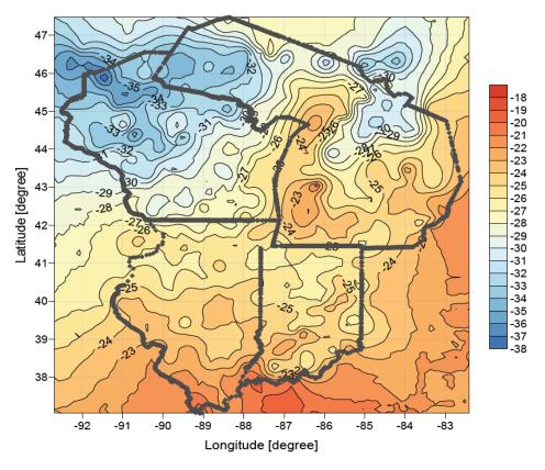
Figure 3-3. Pavement temperature at the surface in the northern part of the US (reliability=98%)
