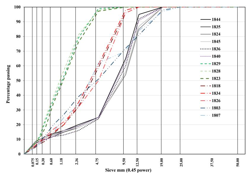
Figure 2-3. Aggregate gradations for the investigated plant-produced mixtures
