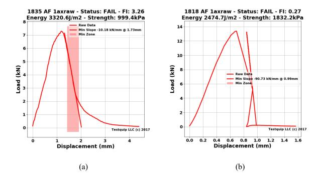
Figure 3-24. Load-displacement response for aged mixtures under I-FIT testing: a)1835 b)1818
