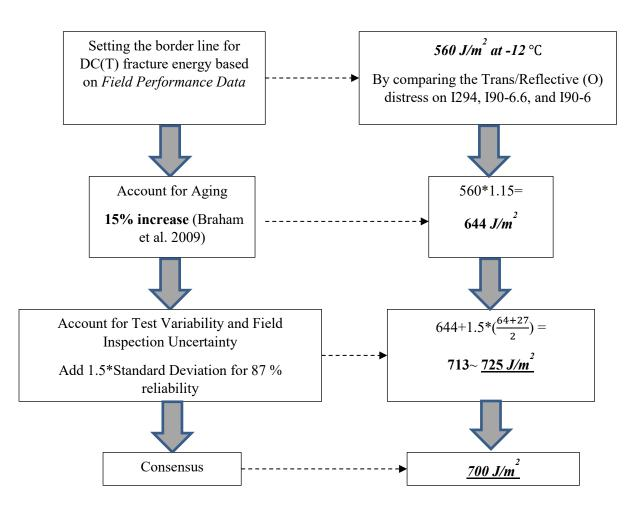
Figure 7-10. Flowchart to Calibrate DC(T) spec for SMA surface mixtures
