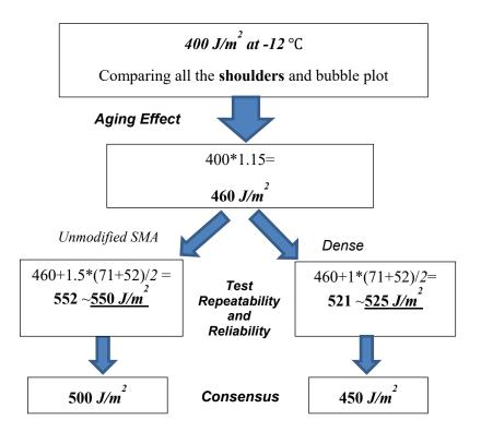
Figure 7-12. Flowchart to Calibrate DC(T) spec for shoulder surface mixtures including "Unmodified SMA", and "Dense" shoulder surface mixtures
