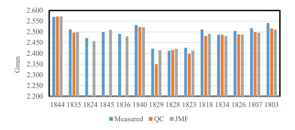
Figure 2-7. Comparing different  $G_{mm}$  values for the studied mixtures (Measured = Test performed in MAPIL; QC = Measured by quality control crew; JMF = job mix formula)
