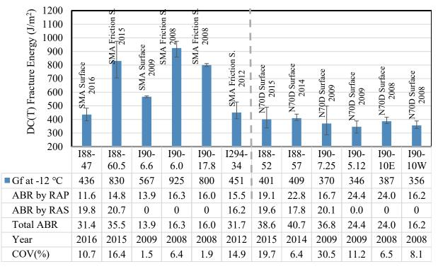
Figure 5-1. DC(T) testing results at -12 °C for the top lift of the field cores
