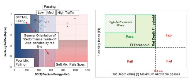
Figure A-9. a) Performance-Space diagram with limits superimposed (W. G. Buttlar et al., 2016) b) Interaction plot for a balanced mix design (Al-Qadi et al., 2015)
