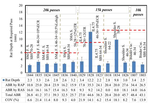
Figure 3-11. Hamburg testing results at required number of passes at 50 °C
