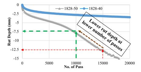
Figure 7-8. Computing a shift in number of passes for 1828 mix
