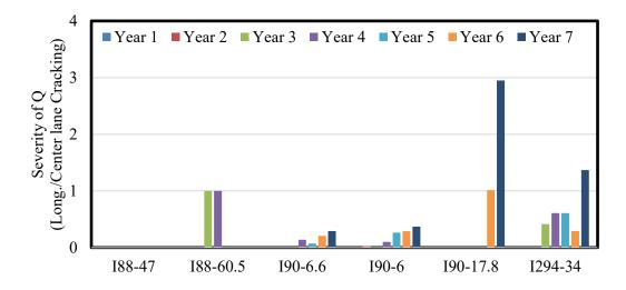
Figure 6-4. Average severity of longitudinal/center lane cracking distress (Q) as a function of service life
