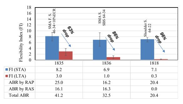
Figure 3-23. Comparing the FI of short-term aged (STA) with long-term aged (LTA) samples
