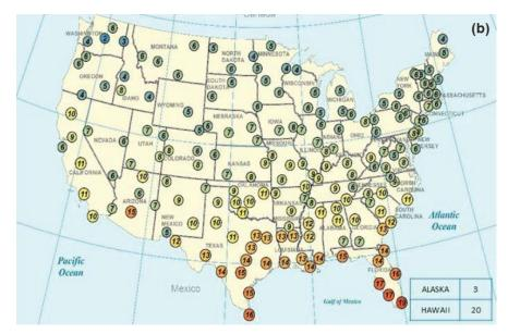
Figure 3-20. Required oven aging durations at 95°C to match level of field aging 6 mm below pavement surface for 8 years of field aging (Kim et al., 2018)
