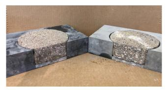
Figure 5-7. Hamburg samples with 12mm PCC shims placed below asphalt specimens
