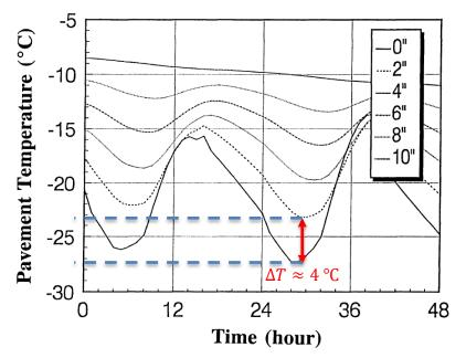
Figure 7-3. Effect of depth on the layer temperature as a function of depth (SHRP A357 Report, 1993- Location: Frazier, Minnesota)
