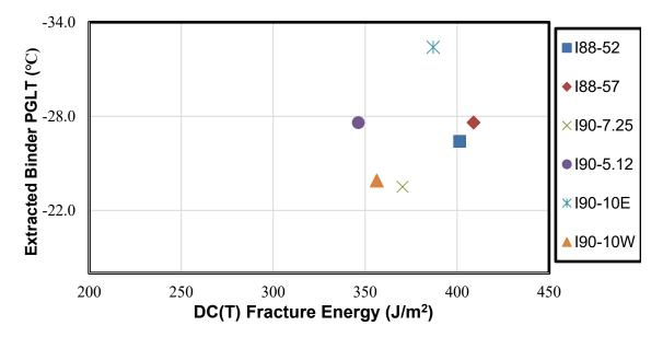
Figure B-5. Comparison between DC(T) fracture energy and extracted binder PGLT for field cores
