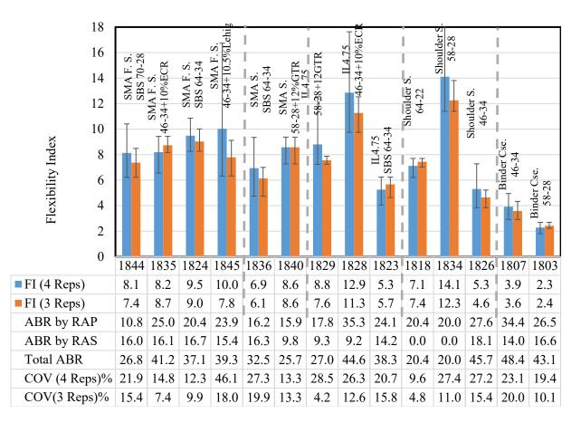
Figure 3-5. I-FIT testing results (four replicates vs. three replicates)
