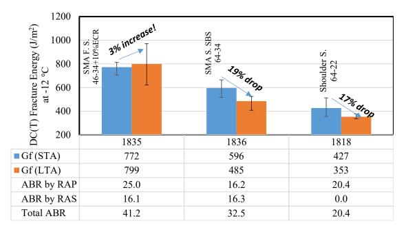
Figure 3-22. Comparing the DC(T) fracture energies of short-term aged (STA) with longterm aged (LTA) samples
