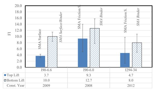
Figure 5-4. Comparing the FIs for top and bottom lifts of the field cores
