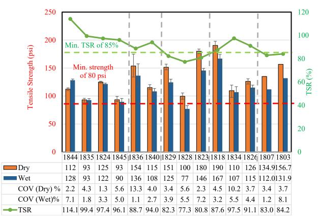
Figure 3-16. Wet and dry strengths and TSR values
