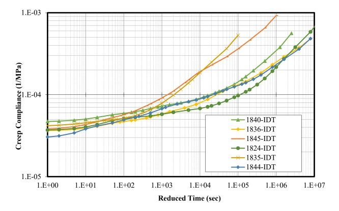
Figure 3-10. IDT creep compliance master curves (Reference temperature: -24 °C)
