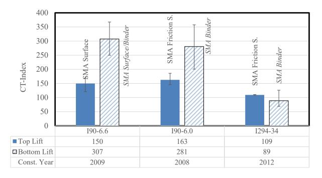
Figure 5-6. Comparing the IDEAL-CTs for top and bottom lifts of the field cores
