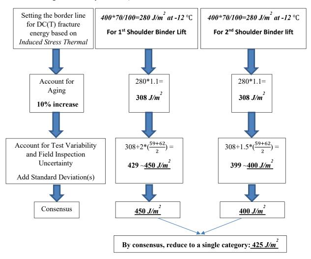
Figure 7-14. Flowchart to calibrate DC(T) thresholds for shoulder binder mixtures
