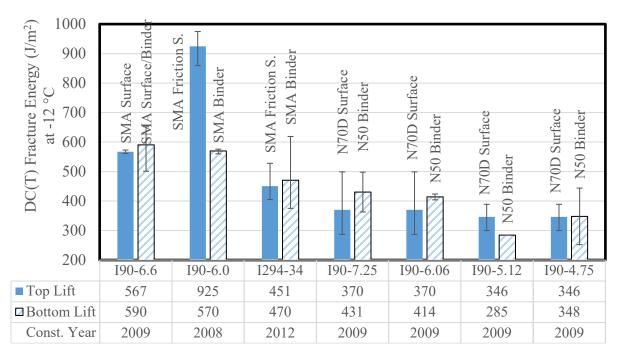
Figure 5-2. Comparing fracture energies for top and bottom lifts of the field cores
