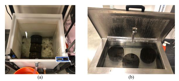
Figure 3-15. TSR sample conditioning. a) Dry set at 25 °C, b) Wet set at 60 °C
