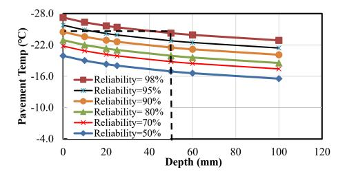
Figure 7-5. LTPP bind software outputs for pavement temperature in winter as a function of depth and reliability in Northern Illinois
