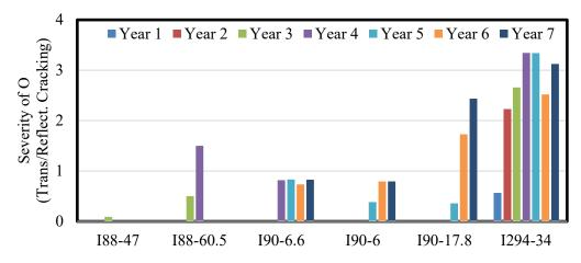
Figure 6-5. Average severity of transverse/reflective cracking distress (O) vs. service life
