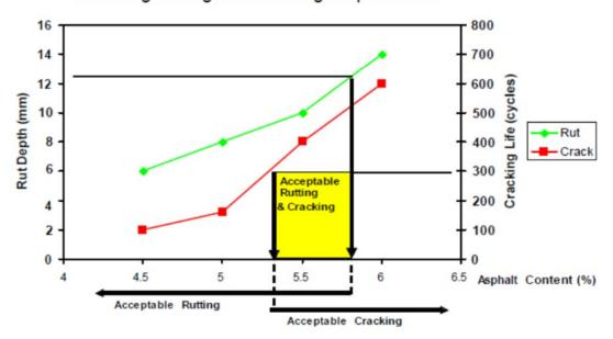
Balancing Rutting and Cracking Requirements
