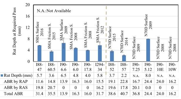
Figure 5-8. Hamburg testing results for the top lift of the field cores
