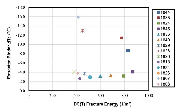
Figure B-2. Comparison between DC(T) fracture energy and extracted binder PGLT
