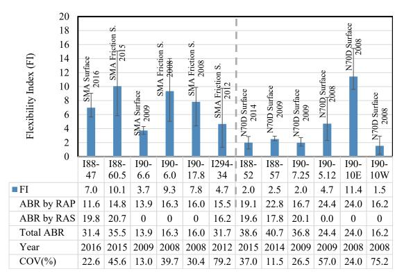
Figure 5-3. I-FIT testing results for the top lift of the field cores
