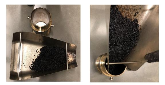
Figure 2-8. Transferring the heated mix to the mold
