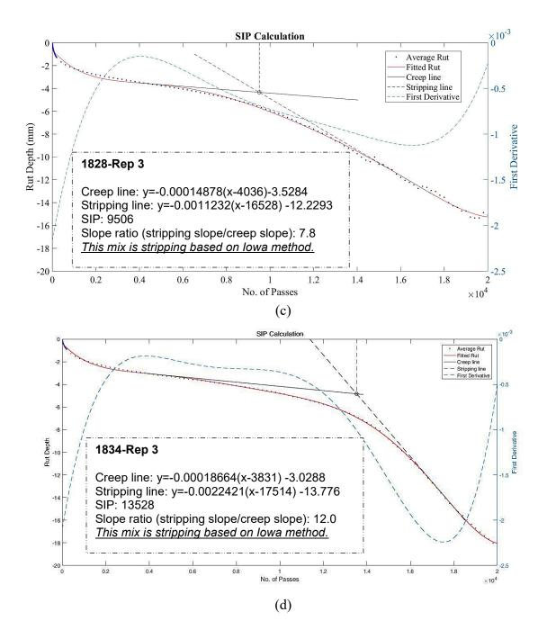
Figure 3-13. Examples of determination of SIP: a) 1835, b) 1845, c) 1828, d) 1834 mixtures
