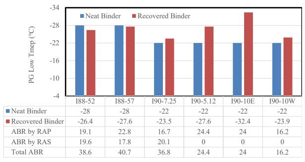
Figure B-4. Comparing PGLT of neat and recovered binders (without further lab aging)
