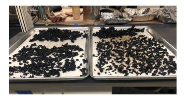
Figure 2-6. Preparing samples for theoretical maximum specific gravity (G<sub>mm</sub>) testing
