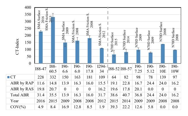
Figure 5-5. IDEAL-CT testing results for the top lift of the field cores
