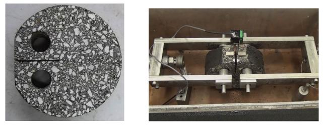
Figure A-1. a) Prepared DC(T) specimen (W. G. Buttlar et al., 2016) b) DC(T) Test setup
