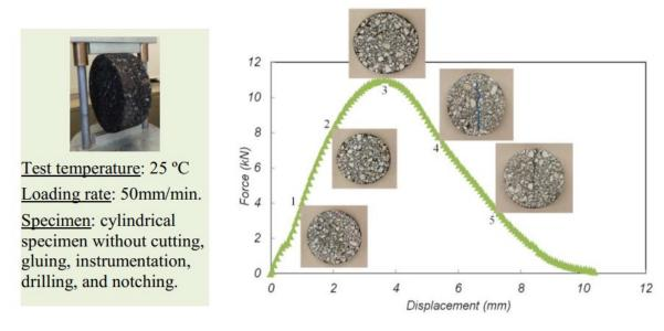
Figure A-6. IDEAL-CT Test Setup and Typical Results (Fujie Zhou et al., 2017)
