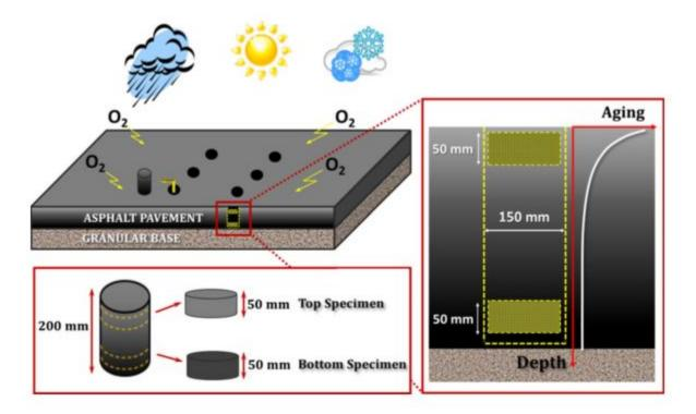
Figure A-8. Schematic representation of pavement aging gradient with respect to depth (Behnia et al., 2014)
