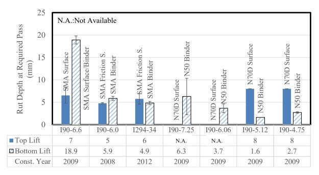
Figure 5-9. Comparing the rut depths for top and bottom lifts of the field cores
