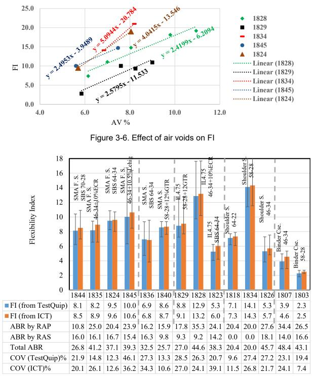
Figure 3-7. Comparing FIs calculated from Test Quip and ICT software
