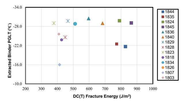
Figure B-1. Comparison between the DC(T) fracture energy and extracted binder PGLT
