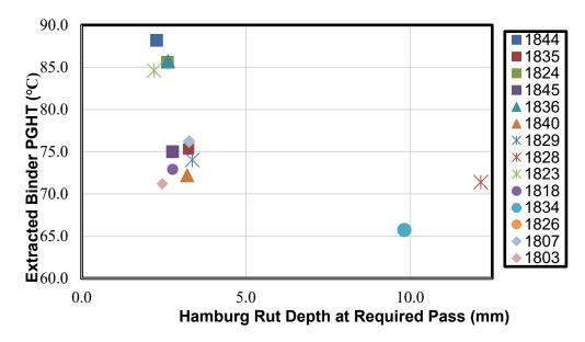
Figure B-3. Comparison between Hamburg rut depth and extracted binder PGHT
