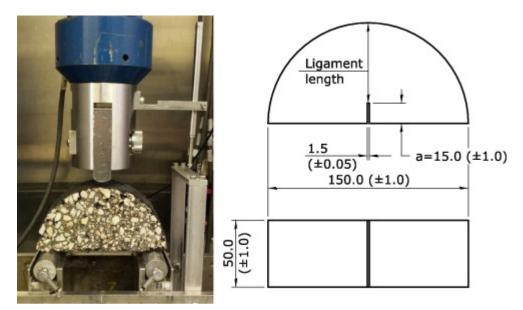
Figure A-3. SCB specimen and test setup (Ozer, Al-Qadi, et al., 2016)
