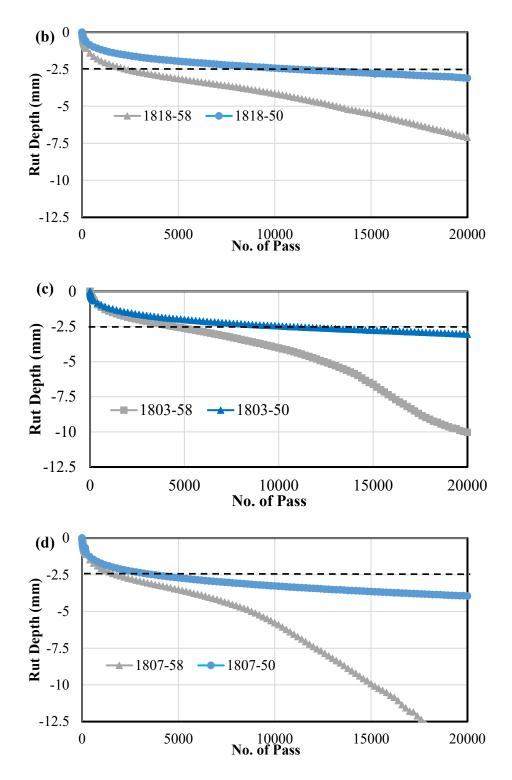
Figure 7-7. Comparing Hamburg testing results at two different temperatures, a) 1829, b) 1818, c) 1803, d) 1807
