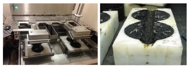
Figure A-7. Hamburg Wheel Tracking Device a) Test running b) After test (W. G. Buttlar & Rath, 2017)
