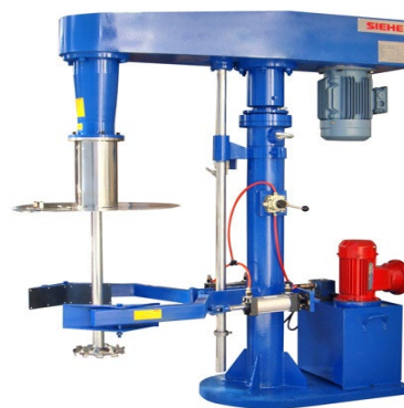
Figure 2: Bench-scale binder-ECR mixing system
